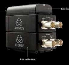
They are stackable too. With the AC power supply included, you can charge up to three Connect units simultaneously.
