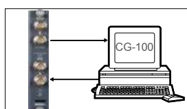
Downstream keyer for Internal and External keying options. Use with Datavideo character generators
