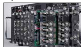
Install optional cards including SDI, DVI, downstream keyer, genlock in and more
